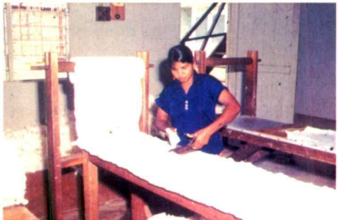
(f) Cutting long sheet to required length
