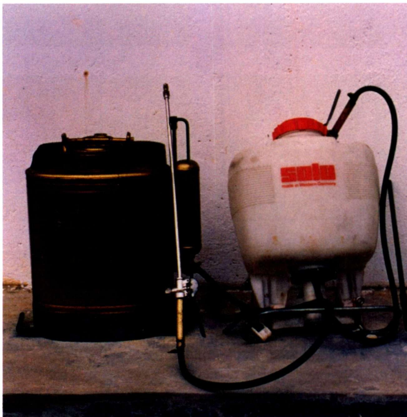
Figure 7.2 Knapsack sprayers of 18 litres capacity - brass (left) and PVC (right)
