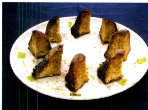
Figure 10.8 Cuplump samples after drying with appropriate setting
