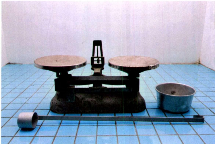
Figure 10.3 Apparatus for the determination of DRC of latex by the dipper or “chee” method
