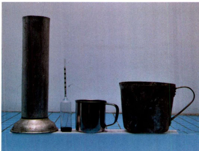
Figure 10.4 Apparatus for the determination of DRC of latex by the hydrometer metrolac method
