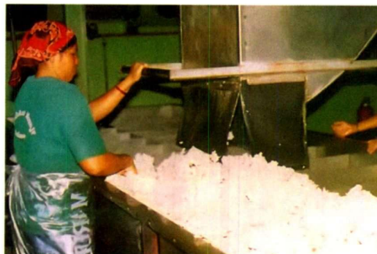
(b) Placing crumbs in dryer box
