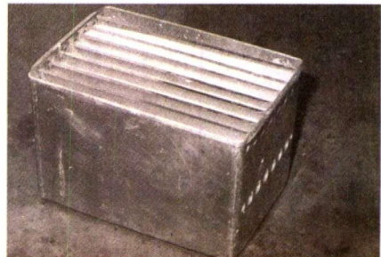
(f) Placing partition plates
