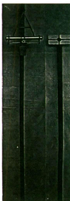
(a) Road tracer and sighting board
