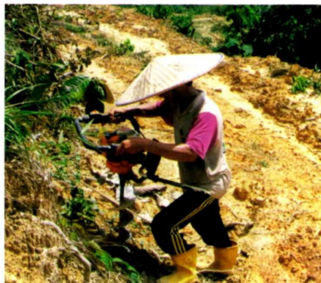
(b) A mechanical digger (soil borer) is used at sloping areas
