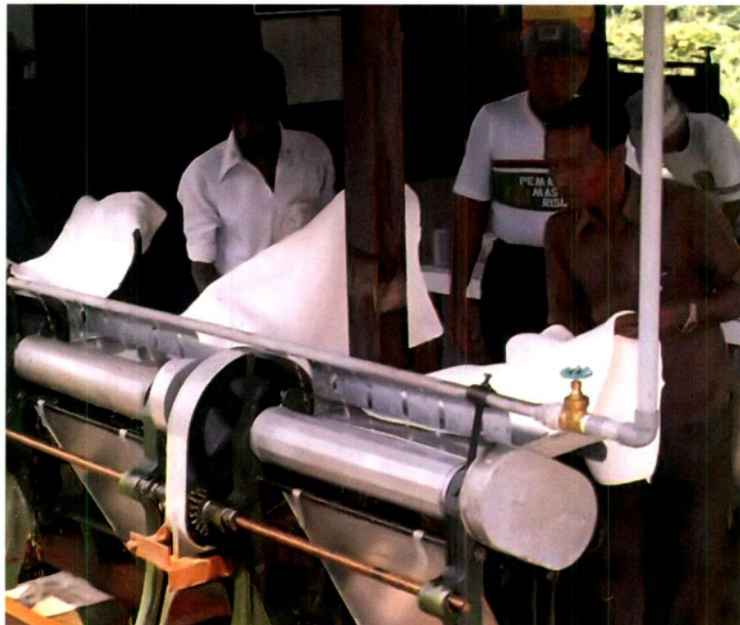
(b) Milling of coagulum through smooth roller on the left and groove roller on the right
